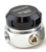
Patent pending OPR T40 is an oil pressure regulation system for turbochargers. It helps prevent compressor or turbine stage oil leaking/smoking and takes the guesswork out of oil restrictor sizing for more efficient and effective oil delivery. The OPR ensures the oil pressure going to the turbocharger never exceeds 40psi, regardless of engine oil pressure. A true plug and play setup for oil feed to turbochargers, restrictors not required.
